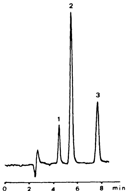
Fig. 3. Typical HPLC separation between benzyl alcohol (1, c = 20.84 mg/ml), methyl paraben (2, c = 20 \mu g/ml) and benzaldehyde (3, c = 13.21 \mu g/ml, equivalent to 0.063% of benzyl alcohol) with UV-282 detection (att. 32). Chromatographic conditions as in Fig. 2.
